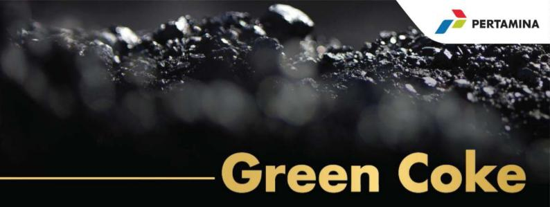
Green Coke, produced in UP II Dumai Refinery, is proceed from solid carbon substance utilizing Delayed Cooking Unit, which is able to be transferred from short residue to Green Coke.
